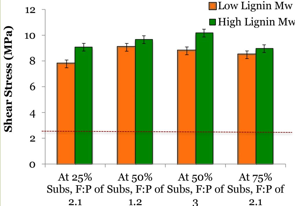
Curing Temperature: 180°C; Pressure: 1.4 MPa
