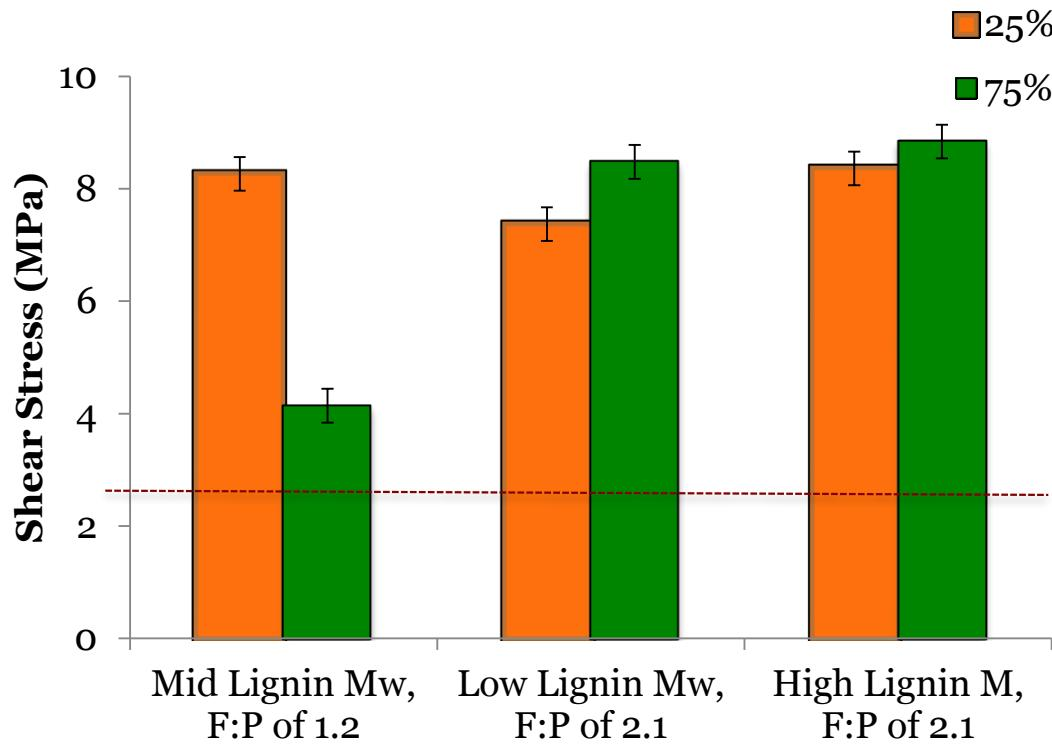
Curing Temperature: 180°C; Pressure: 1.4 MPa
