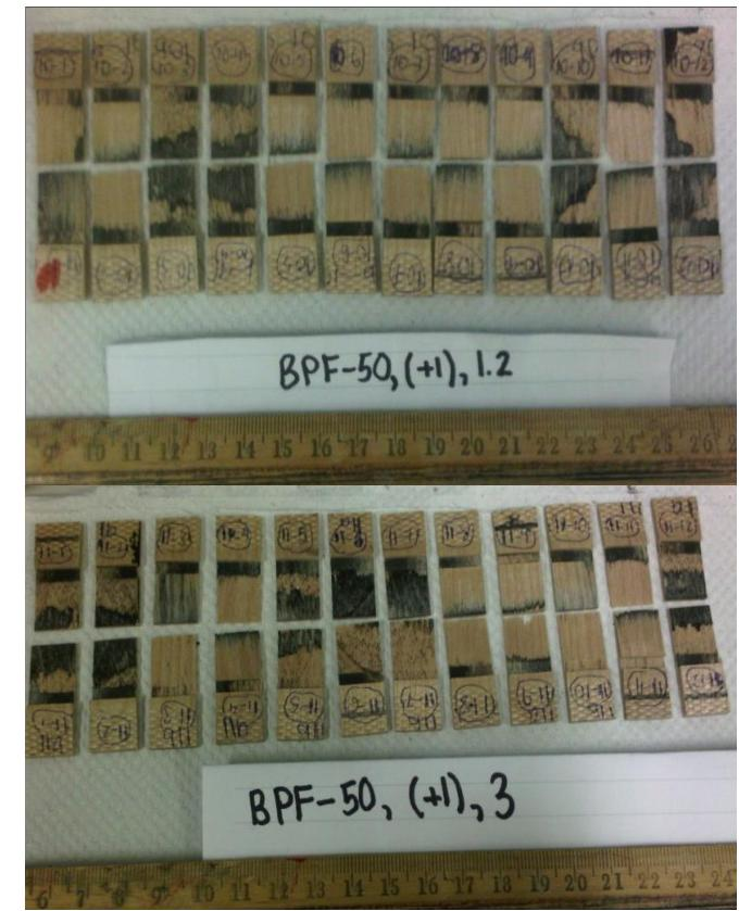
Curing Temperature: 180°C; Pressure: 1.4 MPa
