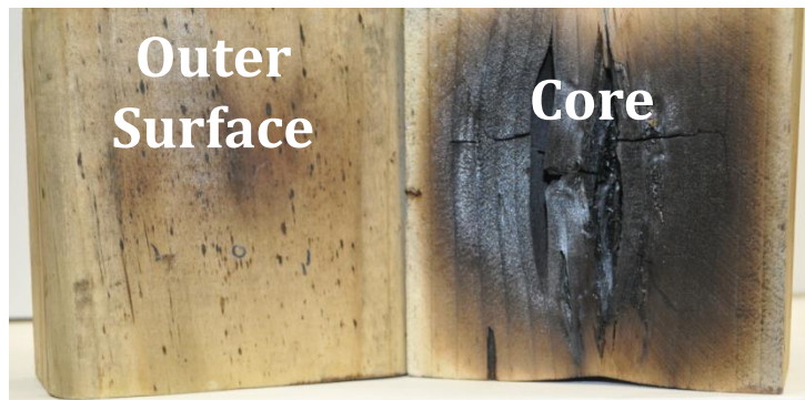
Wood block heated by 2.45GHz microwaves for 360s @ 2.7kW.
