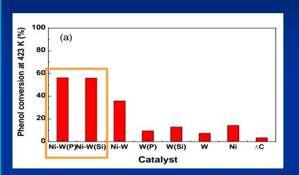
(a) Comparison of the steady-state phenol conversions of different catalysts in HDO of phenol at T = 423K, P = 1,5 MPa and WHSV = 0,5 h<sup>-1</sup>.
