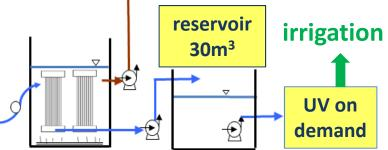
Closed vessel UV-C disinfection system - 2 mercury vapour lamps, 0.08kW each (Biotec)
