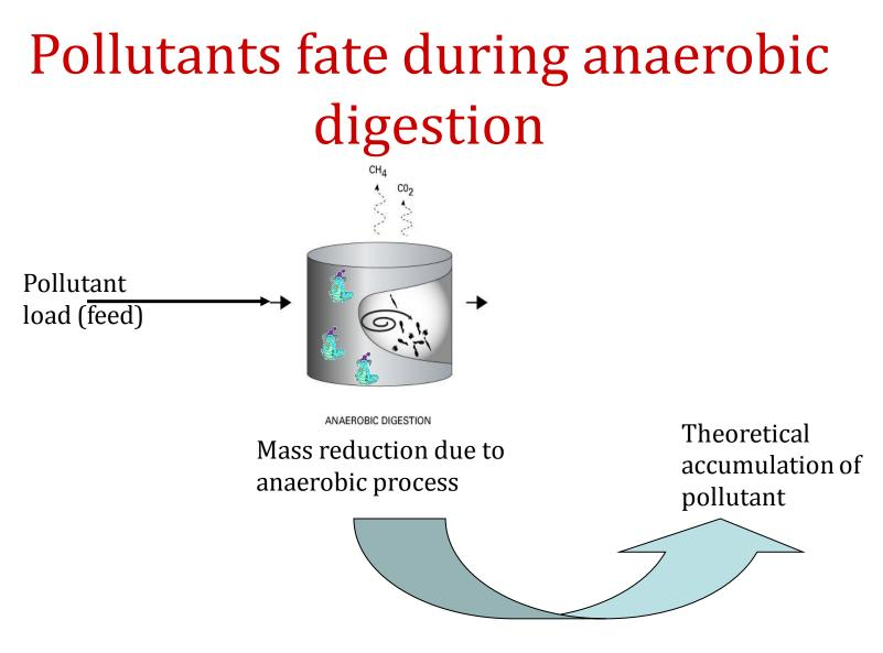
expected concentration in the digested sample: normalized feed concentration with respect to the residual mass
