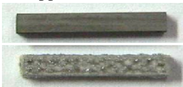
Visual appearance after oxidation
