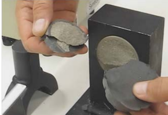
FIGURE 1. Picture of a post shear strength test showing the fractured surface of the composite core
