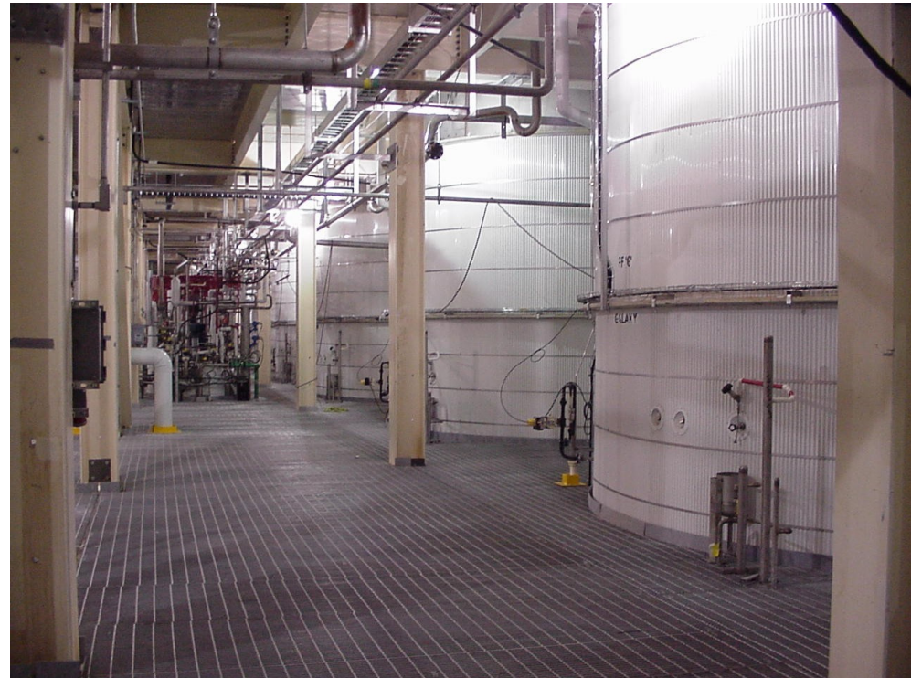
500 m 3 fermenters for lysine production
