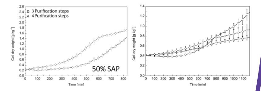
*S. cerevisiae* microscale batch fermentations. 50% (v/v) ( $\Box$ ), 40% (v/v) ( $\bigcirc$ ) and 30% (v/v) dilutions ( $\triangle$ ) of corncob bio-oil aqueous phase (6 purification steps, nylon) (right). No carbohydrates added.
