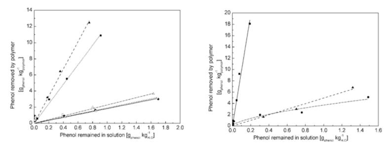
Phenol adsorption isotherms for the textile recycle polymers nylon ( $\blacksquare$ ), polyamide ( $\blacktriangle$ ), PET ( $\odot$ ), cotton balls ( $\triangle$ ) and cotton cloth ( $\bigcirc$ ) (left) and XAD4 ( $\blacksquare$ ), switchgrass ( $\blacktriangle$ ), paper towel ( $\bigcirc$ ) (right).
