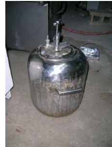
30 L stainless steel batch digester
