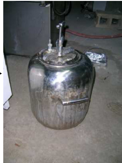
30 L stainless steel batch digester
