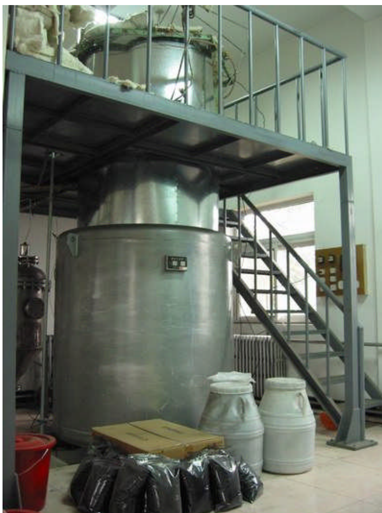
Fig. 4. The pilot plant facility for MWCNT production. [1]
