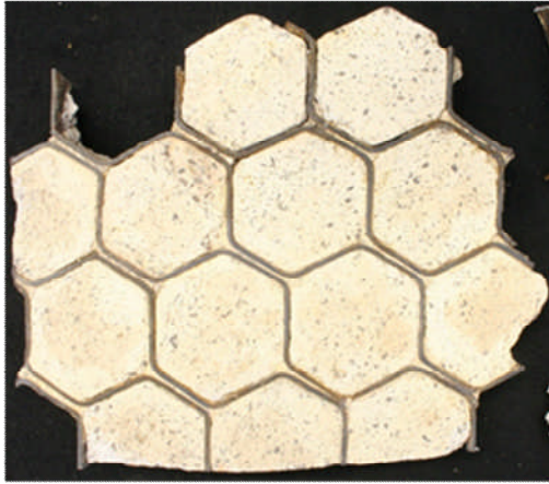
Figure 11: Refractory on process side vs. underside of the hex mesh lining
