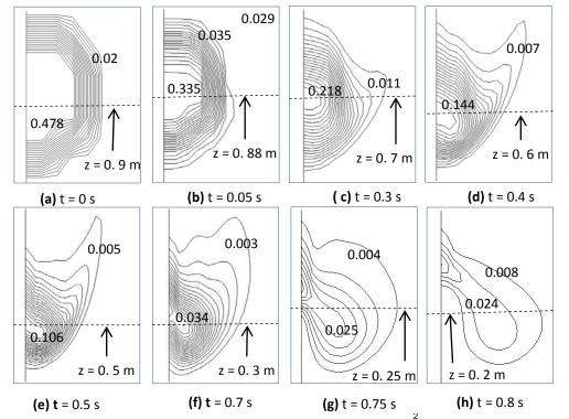
**Figure 2.** Volume fraction of particles at instantaneous time,  $G_s = 10 \text{ kg/m}^2$ .s;  $U_g = 5.5 \text{ m/s}$ ;  $D_{cl} = 30 \text{ mm}$
