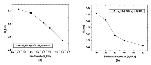
Figure 8. Variation of cluster velocity as a function of (a) Gas velocity and, (b) Solid mass flux at z = 0.5 m
