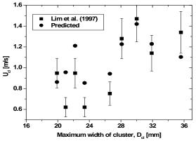
**Figure 7.** Comparison of predicted cluster descent velocity with experimental data of Lim et al. (1997) including 15% error bars,  $G_s = 10 \text{ kg/m}^2.\text{s}$ ,  $U_g = 5.5 \text{ m/s}$ .
