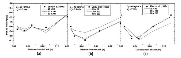
Figure 1. Grid independent test: Lateral profiles of particle velocities for  $D_{cl}$  = 30 mm,  $d_p$  = 213  $\mu$ m, z= 6.2 m, t = 5.2 s]
