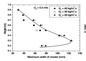
Figure 6. Variation of maximum width of cluster versus height of riser
