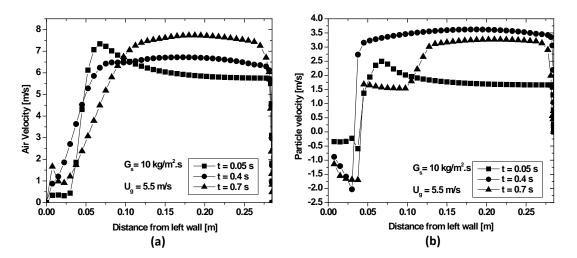
Figure 5. Lateral distributions of (a) Gas velocity and, (b) Particle velocity at z = 0.5 m,  $D_{cl} = 30 \text{ mm}$
