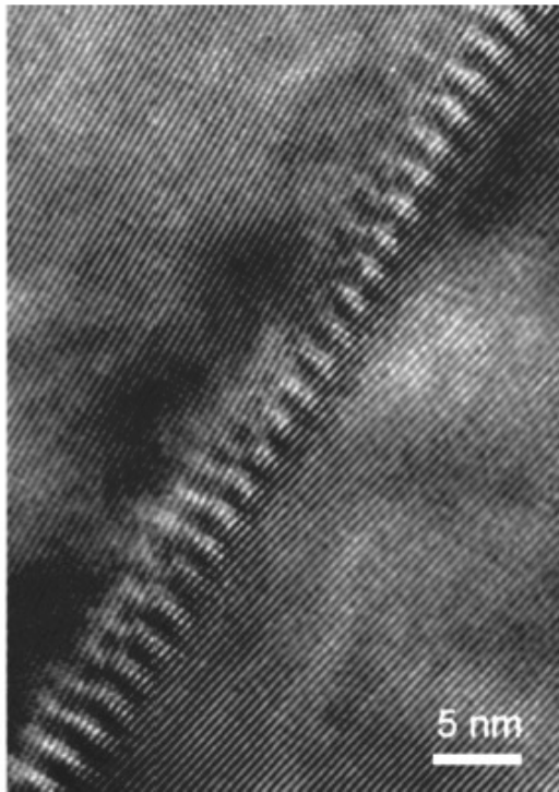
Figure 1. HRTEM of grain boundary in 1.0 mol % Y 2 O 3 -doped CeO 2 . The moiré rings are also visible.
