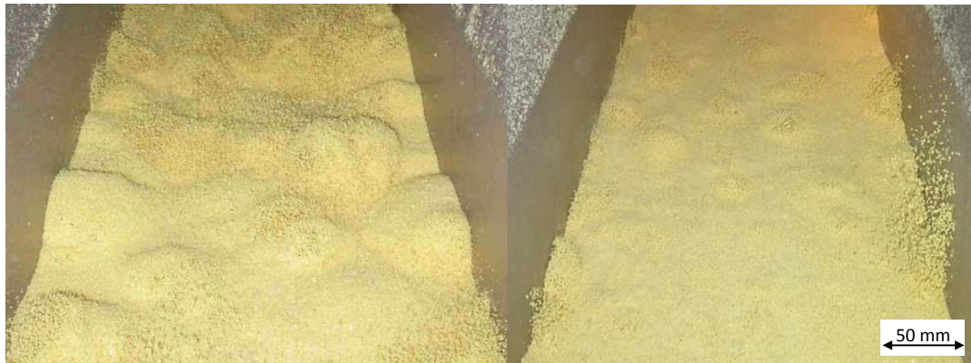
Fig. 1: Different fluidisation states in a continuously operated fluid bed. Left: incipient/minimum fluidisation; Right: bubbling or aggregative fluidisation
