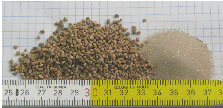
Figure 2. Photograph of biomass particles (left) and glass ballotini (right).
