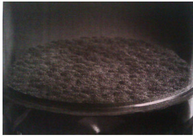
Image 1: photography of the shallow fluidized bed surface for copper beads: 170 \mu\text{m} , n_p=10 (9)
