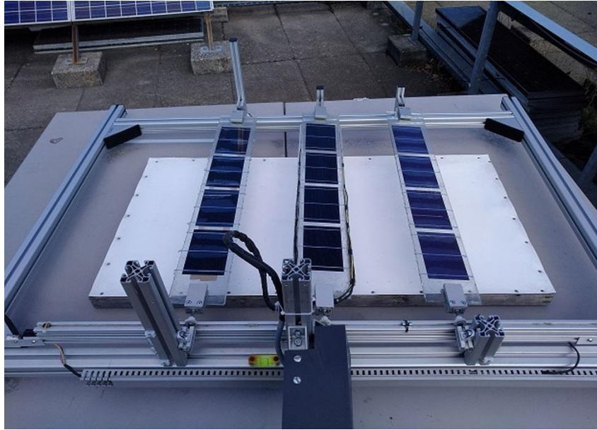
Fig. 3. Miniaturized replica of the BIFOROT array with permanently turning mini-modules at 0^\circ tilt angle. In this configuration the same white reflecting foil as in figure 2 is placed below the mini-modules.
