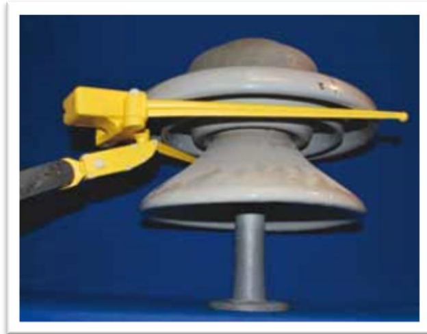
Fig. 2.3. CIAP feelers probing a 120 kV insulator shed [39].
