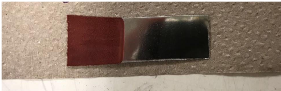
Figure A.2 Cu deposition on the surface of stainless steel electrode
