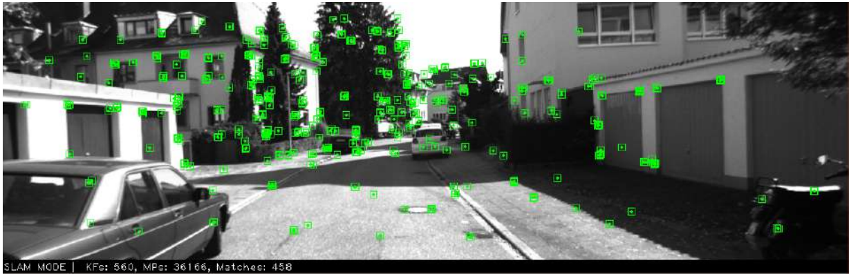
Figure 7.2: A feature extraction on an image by ORB SLAM.
