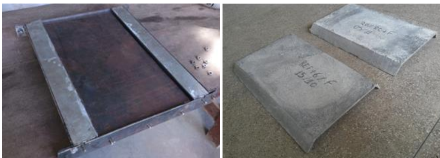
324 325 Fig. 6. Production of SSFRC block: a) metallic mold; b) blocks with natural and recycled aggregate
