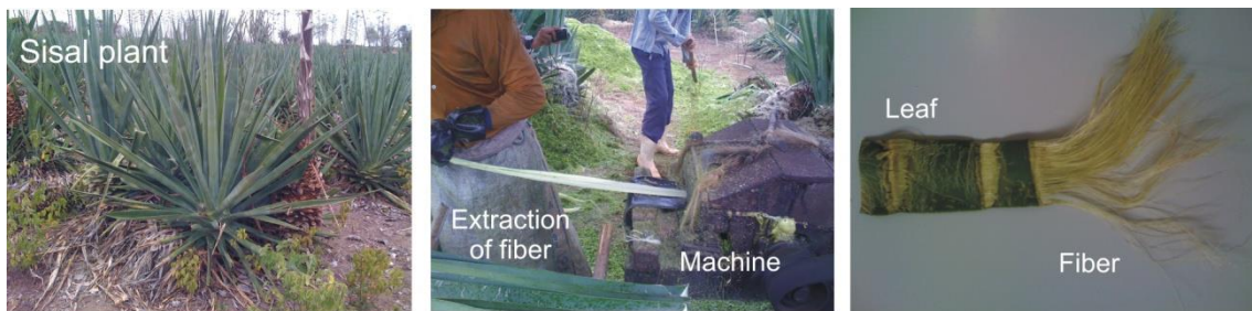
153 Fig. 1. Extraction of vegetable fiber: a) sisal plant; b) fiber decortification process; b) identification of 154 sisal fiber in leaf
