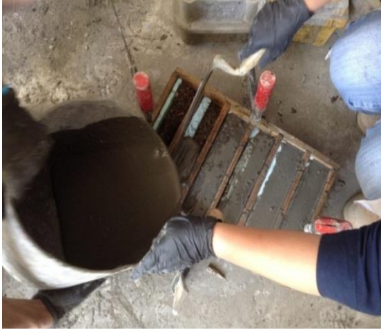
Figure 2. The technique used for producing RSFRM panels
