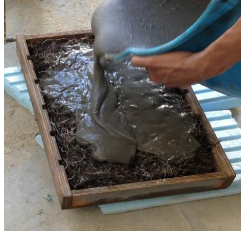
Figure 2. The technique used for producing RSFRM panels
