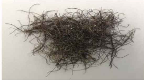
Figure 1. Recycled steel fibres extracted from post consumed tyres
