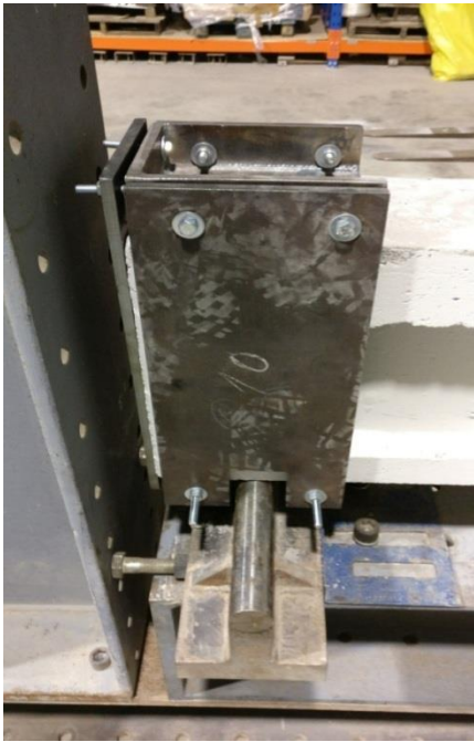
Figure 11. Confinement system applied to the support regions of the RC beams
