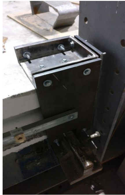
Figure 11. Confinement system applied to the support regions of the RC beams
