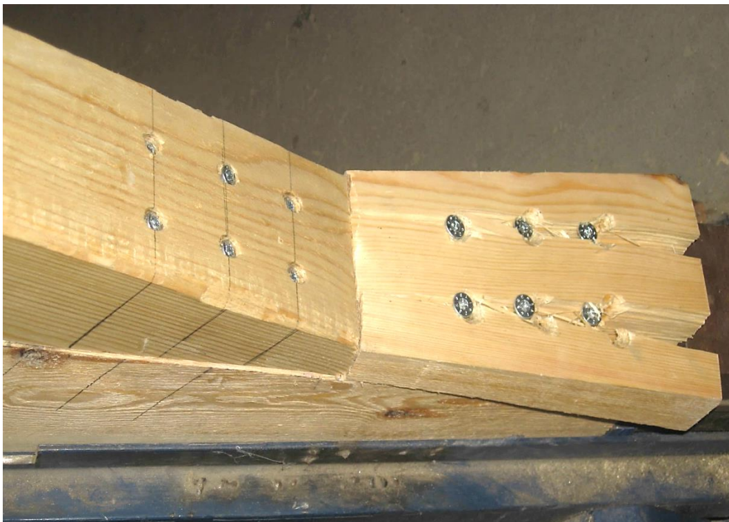
Fig. 12 Shear row splitting in the upper part of the tie beam retrofitted with PTS.
