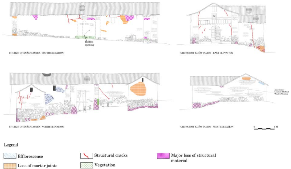
Figure 4. Damage maps in each facade [Zanotti 2015].
