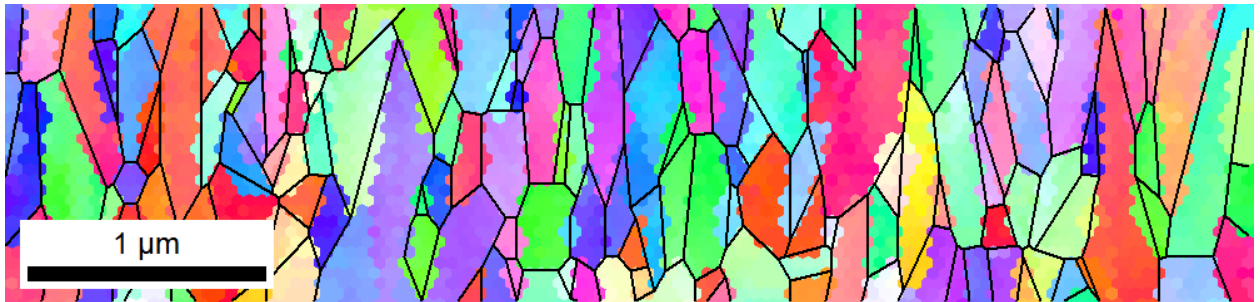
Figure 8 - EBSD results for CrN layer of sample 1.1: unique grains colour map with reconstructed boundaries.
