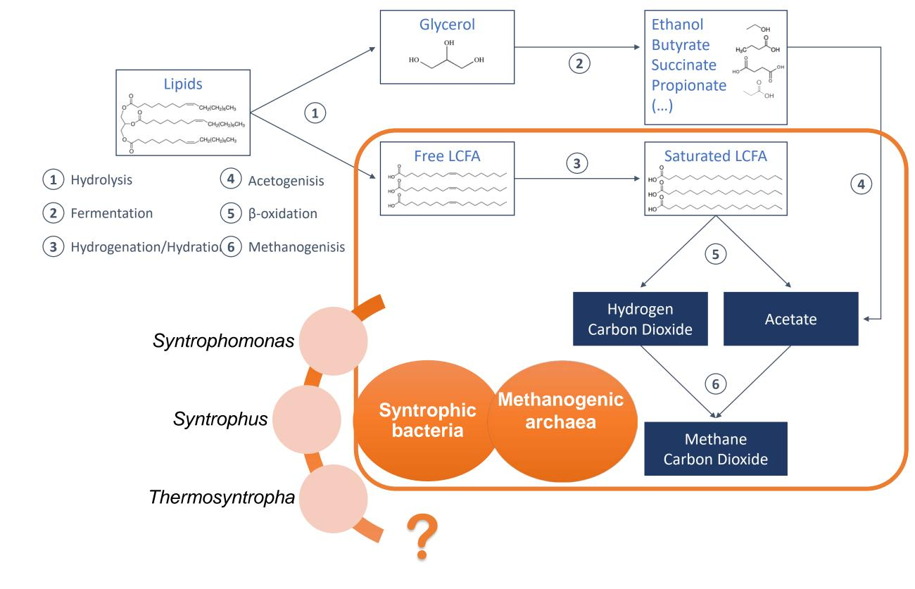
**β-oxidation**: the suggested route for Lipid degradation
