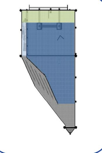
IASB, reactor operated in downflow mode, utilises the flotation as sludge retaining mechanism, and the promotes contact between feed and settled biomass for improving
