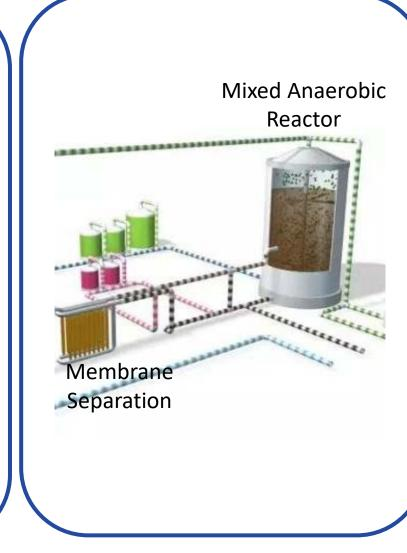
**MEMTHANE**®, by Veolia, retains the biomass inside the reactor by using a membrane coupled to the anaerobic digester/ reactor.
