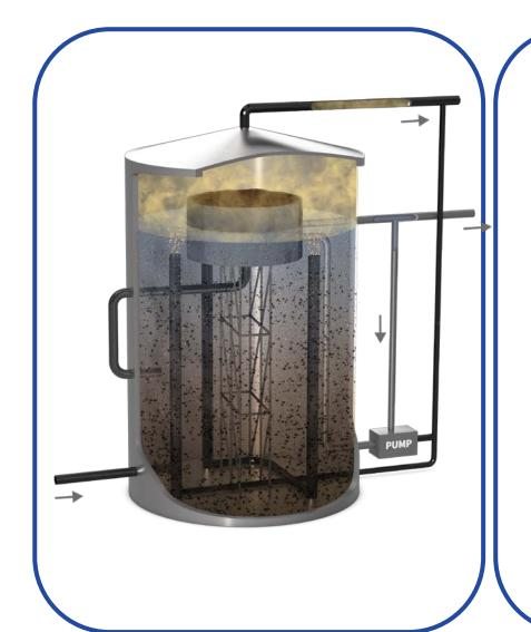
**BIOPAQ®AFR**, utilises Paques, flotation integrated where solids and fats are floated using biogas, and are recirculated back into reactor for further digestion.
