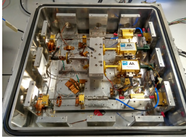
Fig. 21 Assembly of the front-end part for the test inside the cryostat
