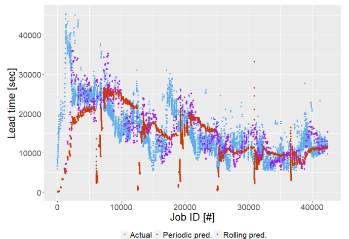
Fig. 2. Job lead times with finite interval Little's law (job type A): actual LT values, one-day periodic and one-day rolling horizon prediction
