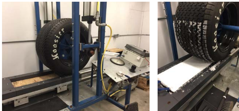
Figure 2.3 Automated trafficking machine used for simulating vehicle traffic in the laboratory
