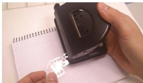
Figure S10. Preparation of the sensory discs by cutting 5 mm diameter circles from the sensory membrane or film Mem with an office paper punch.
