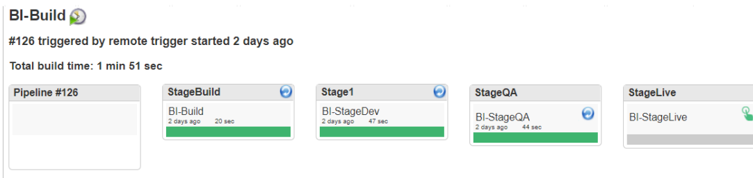
Figure 16 - Pipeline after success of the first three stages
