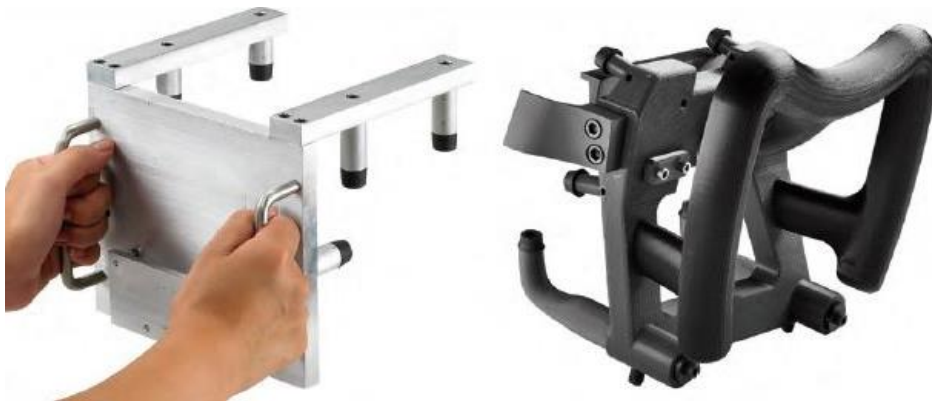
Figure 26 - On the left conventionally machined aluminium fixture for testing bumper support by BMW and on the right 3D printed with ABS thermoplastic fixture [33].
