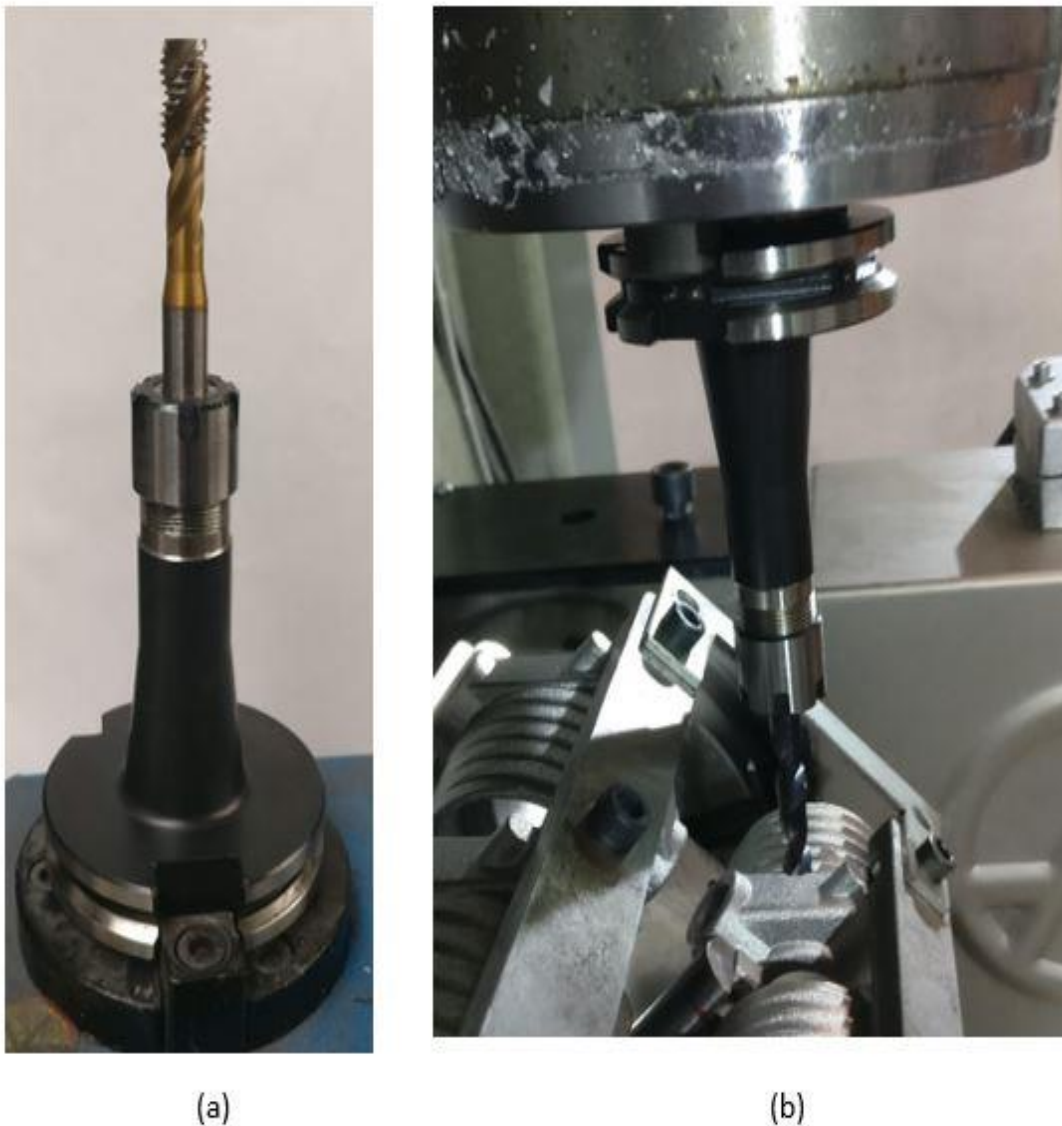
Figure 90 (a) New tool holder of SK 40 specification (b) New tool holder used in finding Z-levels for machining.
