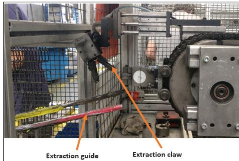
Figure 151 - Extraction claw and extraction guide of TEC 5
