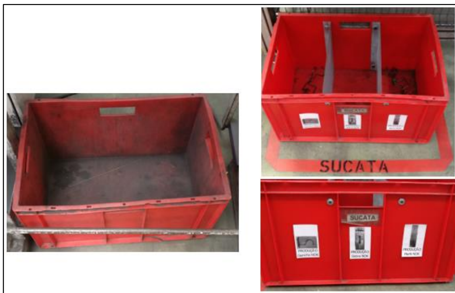
Figure 186 - Scrap container before (left) and after implementation of compartments according to the type of defect (right)
