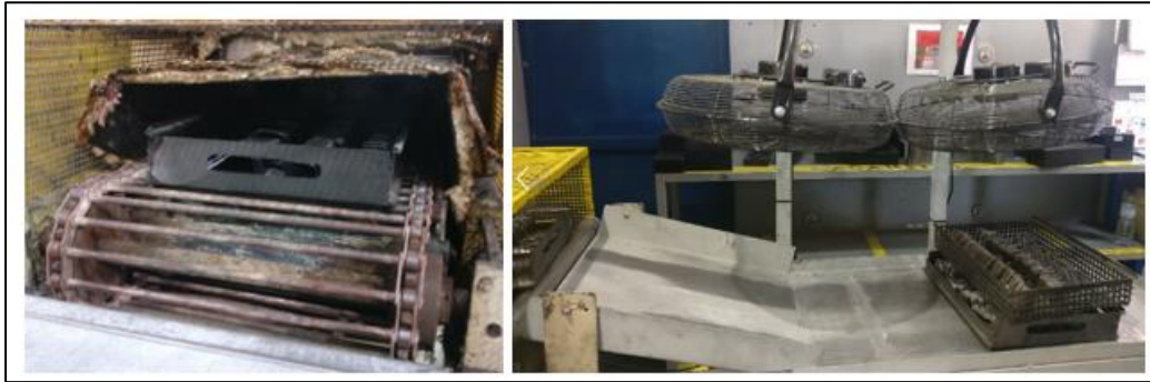
Figure 153 - Entrance of conformed wires in furnace (left) and cooling operation after the heat treatment (right)
