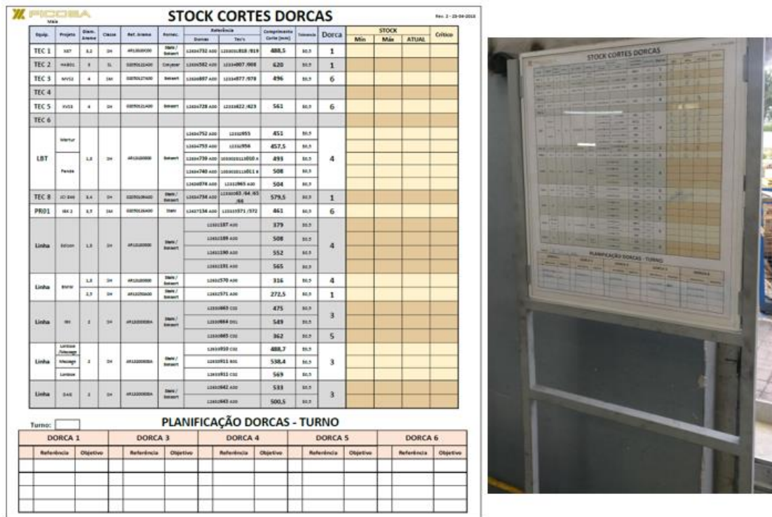
Figure 181 – Dorca equipment stock management board template (left) and presence on the gembra (right)
