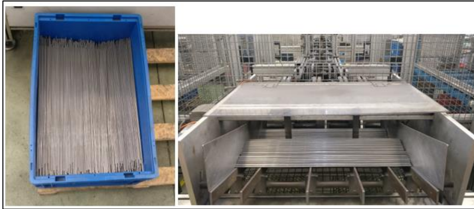
Figure 147 - Container with wire cut by Dorca machines (left) and wire feeding in TEC machine (right)
