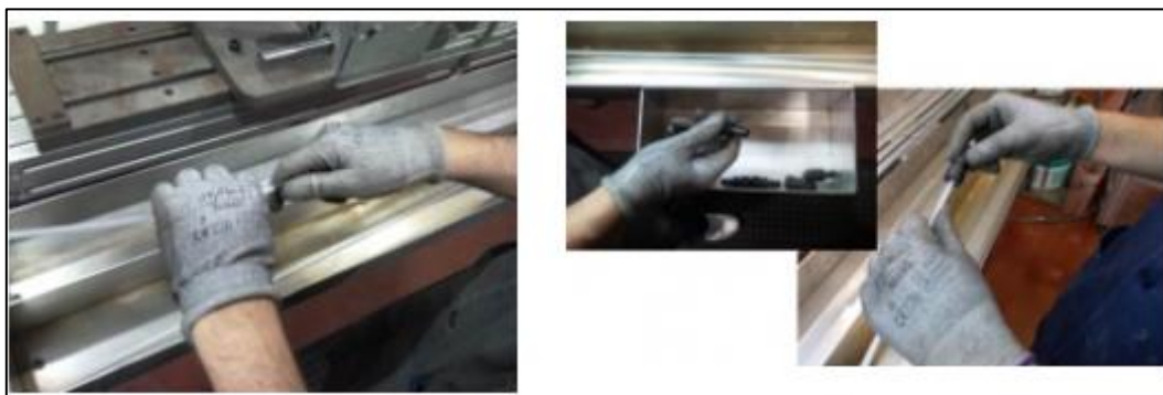
Figure 63 - Assembly of the inner tube on the conduit (left) and insert of the conduit end fitting subgroup into the bigger inner tube (right)
