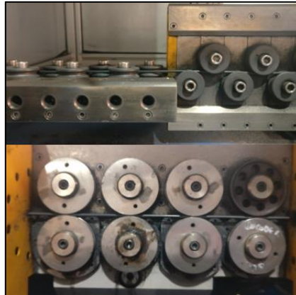
Figure 132 - Straightening rollers (above) and traction wheels (below)
