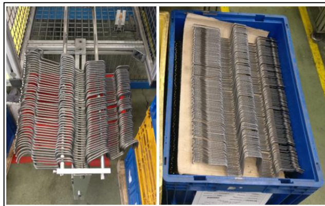
Figure 152 - Conformed wires on the extraction guide of a Dorca machine (left) and on containers to proceed for the next operation (right)
