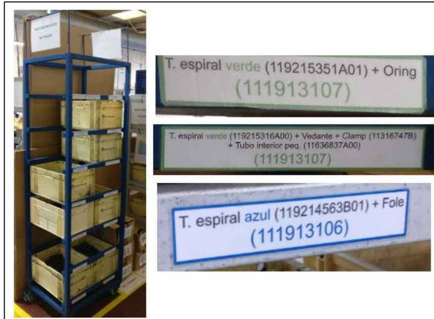
Figure 81 – Conduit end fitting subgroups rack and visual standard used (After)
