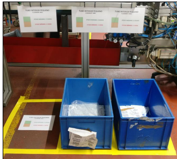
Figure 95 - Small inner tubes stock zone and corresponding visual help added (after)
