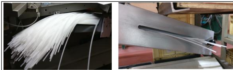
Figure 76 - Bigger inner tube stock container capacity maximized (left) and shape handle to adapt the depth of the container (right)
