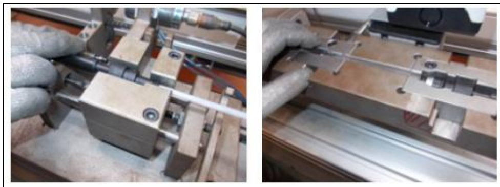
Figure 69 - Operator inserting the cable subgroup on the measurement jig (left) and on the essay jig (right)
