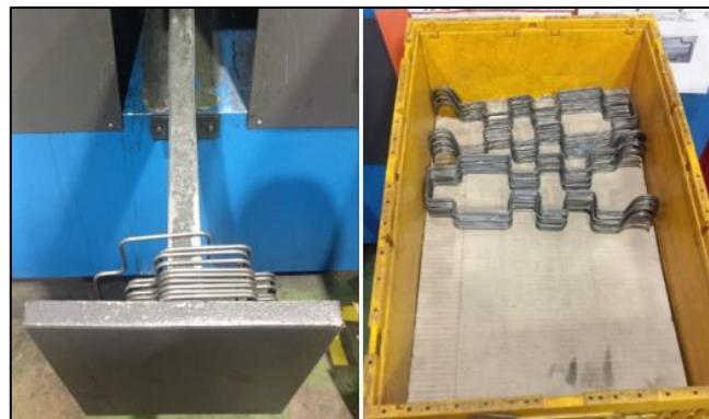
Figure 139 - Wire cut on the extraction guide (left) and wire placed in containers (right) ( Inovmaq )
