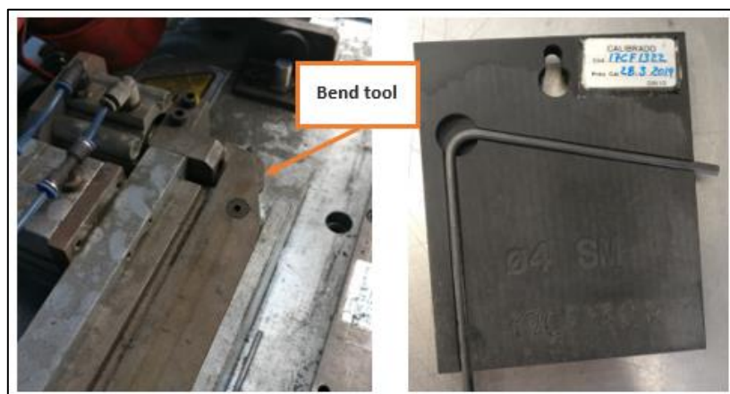
Figure 185 - Wire bending tool of the control workstation (left) and wire bend jig (right)
