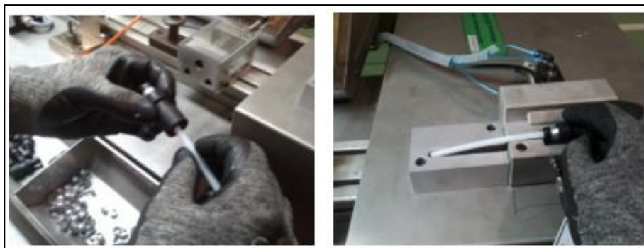
Figure 58 - Assemble of knurled inner tube on the conduit end fitting (left) and final validation of (right)
