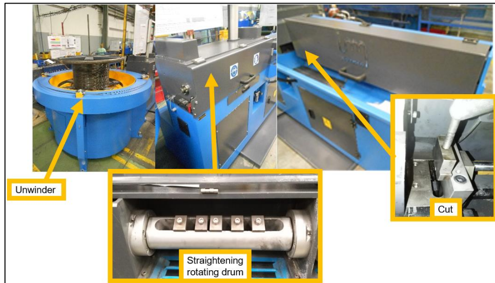
Figure 140 – Wire straightening and cutting process of Dorca machines
