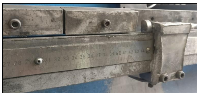
Figure 144 – Length of cut sensor ( Dorca machine)
