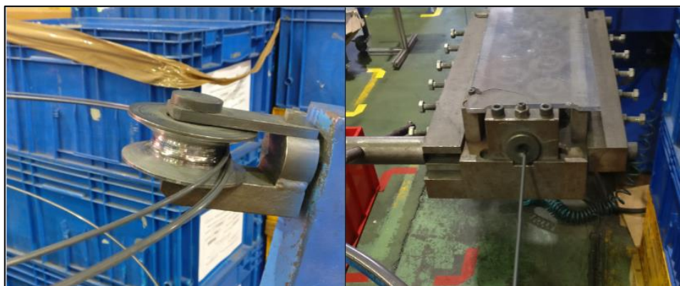
Figure 131 - Unwinder pulley (left) and wire entrance in the CNC bending machine (right)
