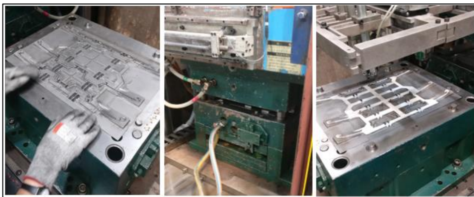
Figure 157 - Operator placing conformed wires in the mold (left), injection operation occurring (middle) and product after injection operation (right)
