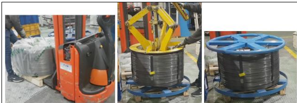
Figure 129 – New wire reel (left) and wire reel being moved to an unwinder support through a mobile bridge (middle) and wire reel mounted on the unwinder support (right)
