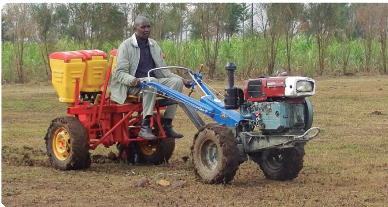
Figure 4.3. Two-wheel tractor equipped with a no-till seeder.
