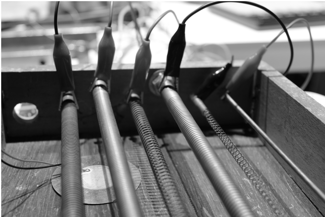
Figure 52: Springs connected to a Makey Makey to control the orchestra.
