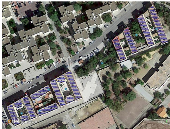
Figure 88: Example of layout of the district in Helioscope : south orientation in the flat roofs.
