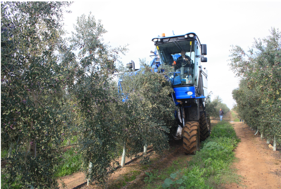
Figure 1.2: Super-high-density olive orchard mechanical harvest in the study area (Sanabria orchard).
