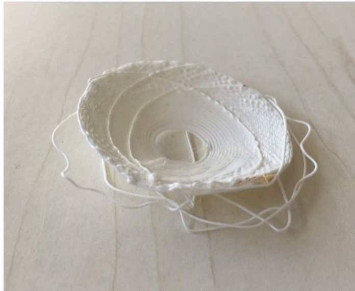
Figure 25 - Damaged model with \alpha=19^\circ printed in Prusa.
