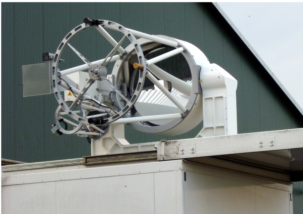
Figure D.9: Scanner unit of the Hohenheim-DIAL, essentially consisting of a small sending telescope, a big receiving telescope, as well as safety devices (radar, camera, and sun detectors).
