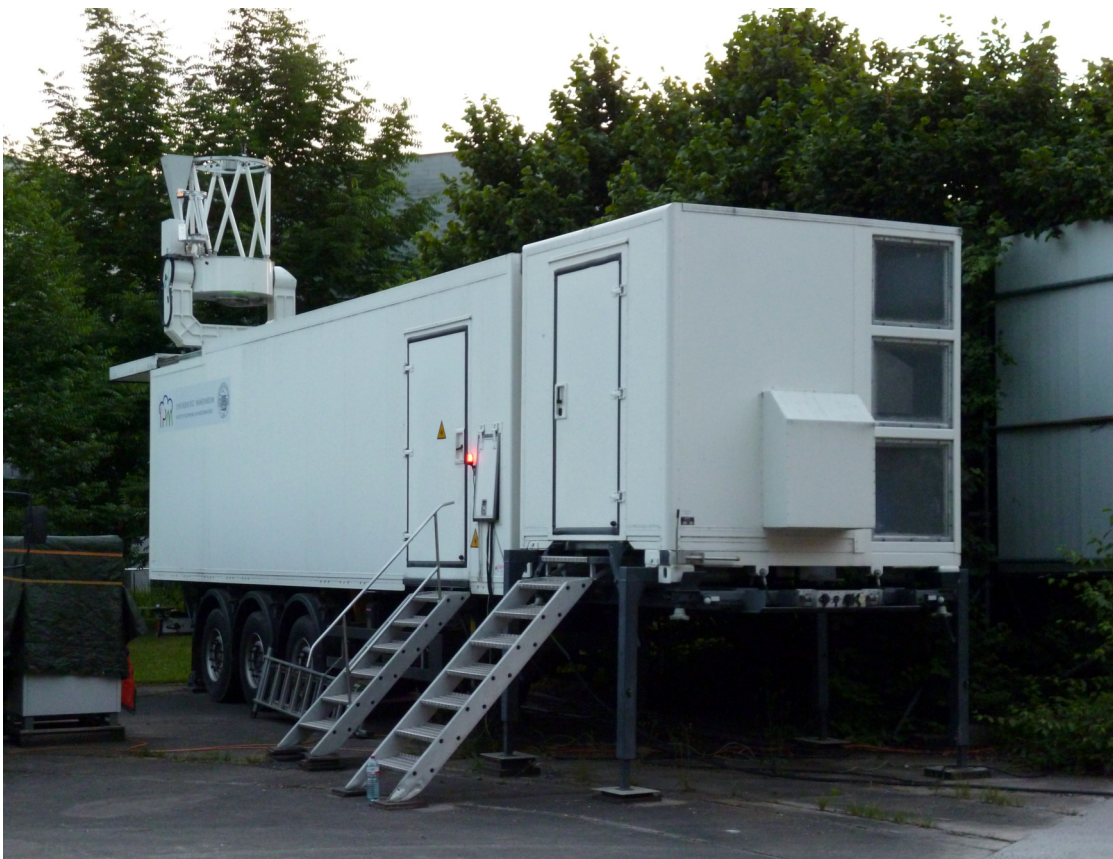
Figure D.1: The water-vapor DIAL of the University of Hohenheim . The energy compartment in the front is decoupled from the rest of the trailer. The main compartment comprehends the laboratory and the scanner room in the rear part.
