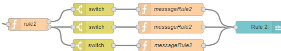
Figure 5.20: Node-RED blocks for the implementation of Nelson rule's Rule 2.
