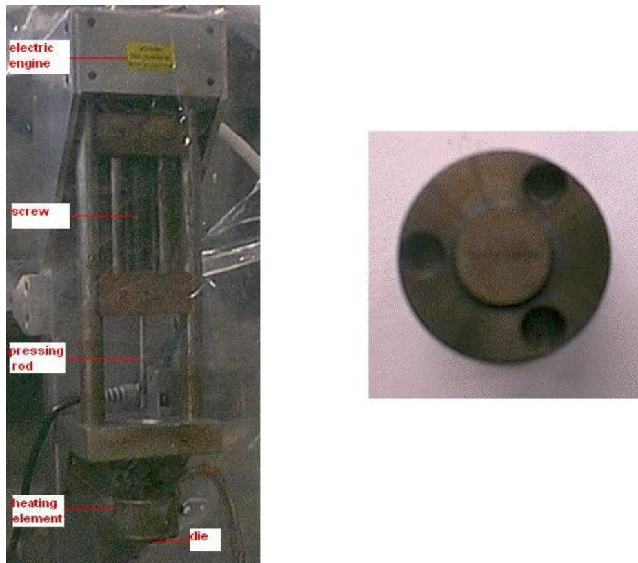
Figure 2-3. Tape-extruder (on the left-hand side) and detail of the die (on the right-hand side) used for the production of samples.
