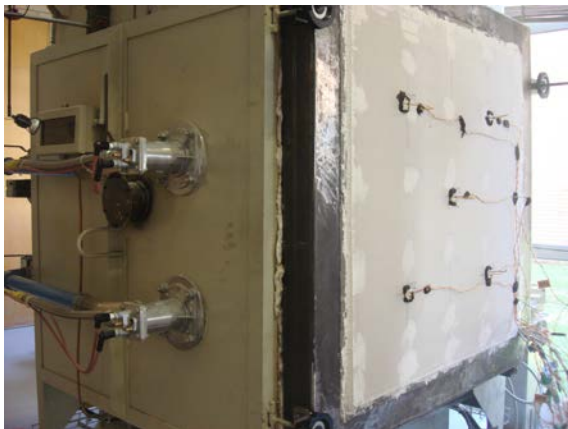
(a) Furnace with the frame attached.
