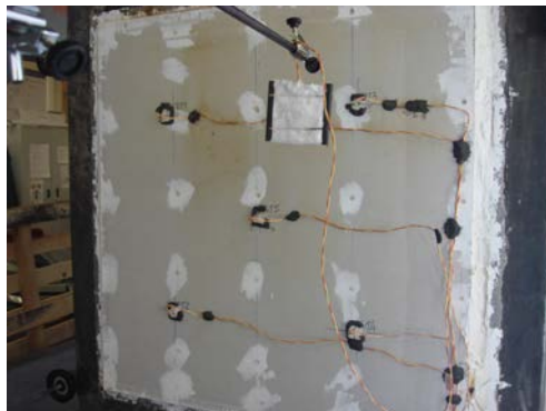
(b) Specimen 0, with emphases for the Disk Thermocouples and the Ambient Thermocouple.
