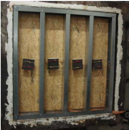
(a) Cavity in Specimen 7.
