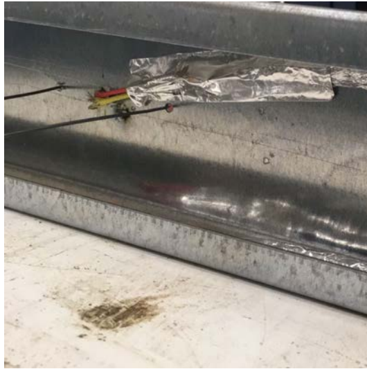
(b) Welded Thermocouple.
