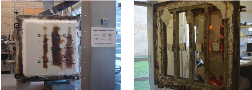
(a) The unexposed side after the end of the test. (b) The exposed side after the end of the test.
