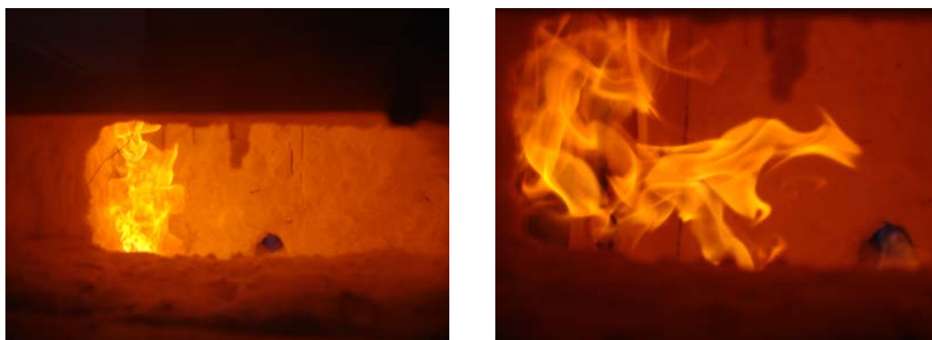
(a) Cork starting to burn through the crack. (b) Cork burning after the fall of the layer.
