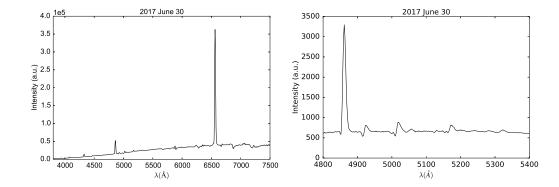
**Figure 4:** Left: spectrum of ASASSN-17hx secured during the rise to the plateau; right: the H $\beta$ , Fe II (42) region
