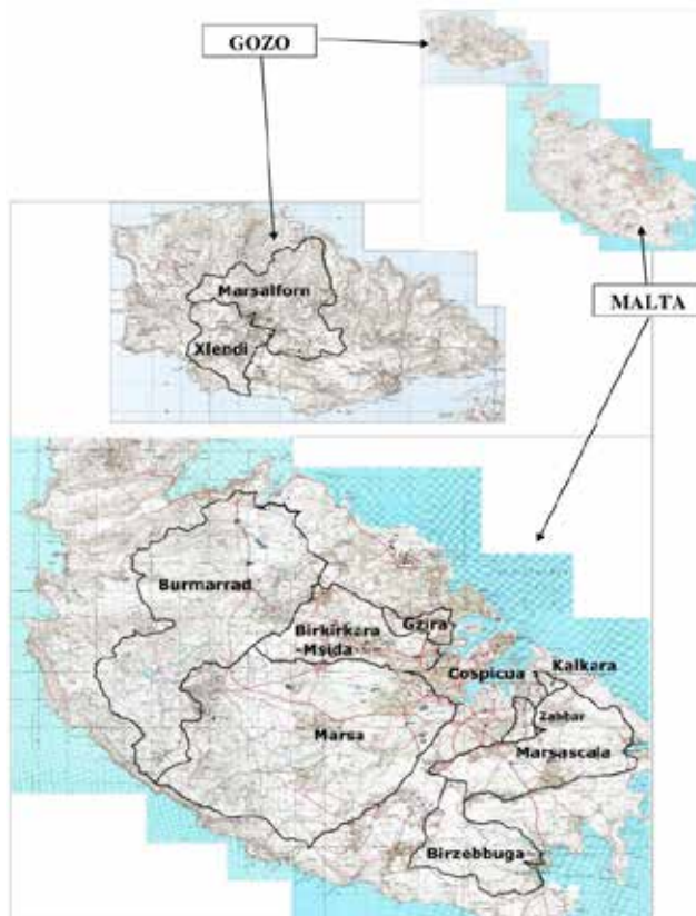
Figure 1: Watersheds as designated in the STWP which are prone to flooding
