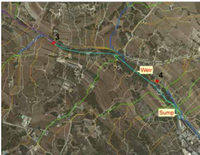
Figure 9: Diversion of stream network into the valley bed and along man-made hydrological features. The edited route is shown in light blue.
