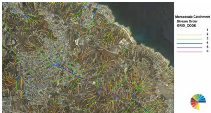
Figure 4: Stream networks derived from the LiDAR data for (a) Marsascula (b) Birkirkara-Msida (c) Gzira (d) Marsa catchments
