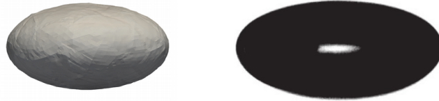
Figure 4.7: (Left) Bubble shape for Eo = 4.88 , \log M = -4.9 . (Right) Experimental bubble shape by [41].
