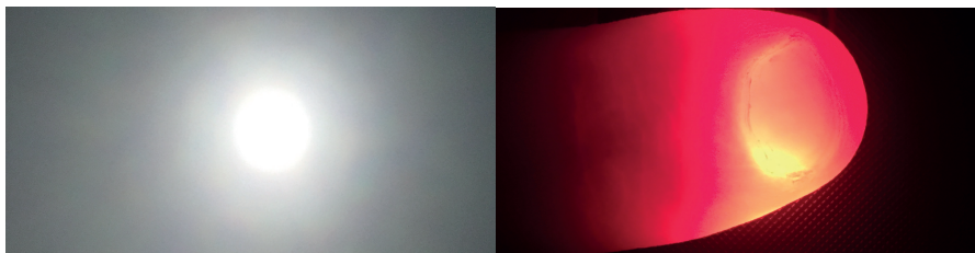
Figure 2.1: Illustrative image: A standard smartphone flashlight (left side) serves as a white light source. Placing a finger on top (right side) illustrates the basis of diffuse optics.
