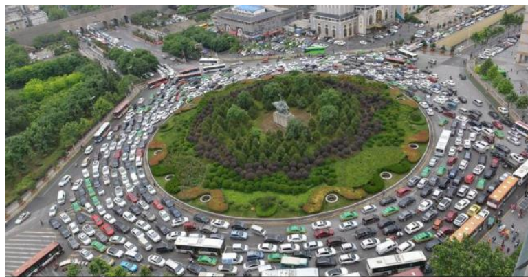
Picture 4. Saturated roundabout
