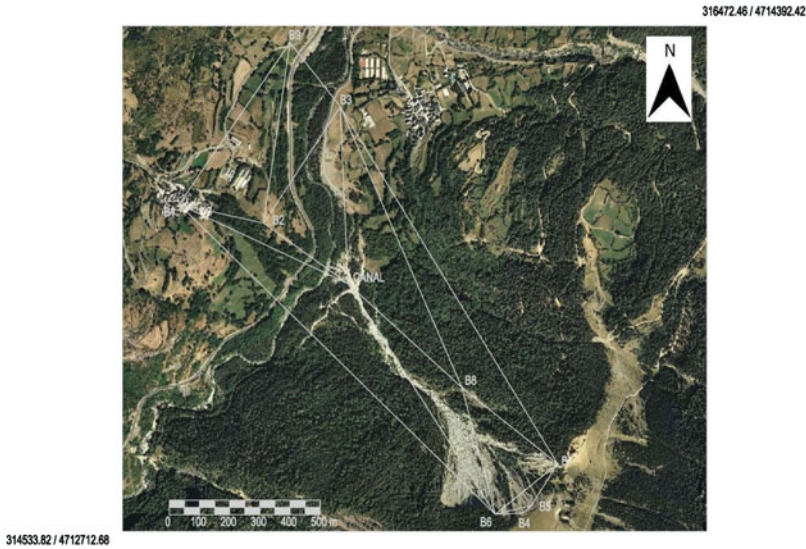
Figure 3. GPS network established in the area to obtain coordinates of the targets and ground control points.
