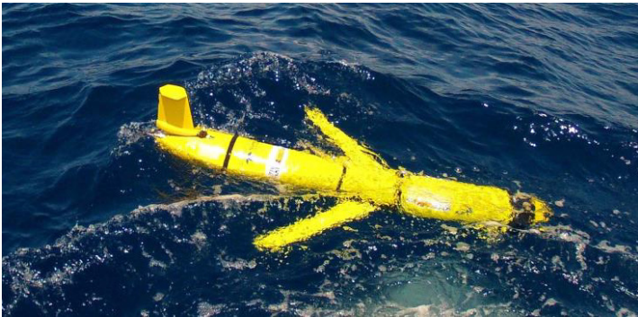
Fig. 2. Buoyancy-driven glider technology example (Slocum G2. Teledyne Marine).
