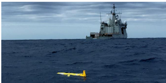
Fig. 5. Glider recovery-maneuver from "Meteoro" patrol-boat.
